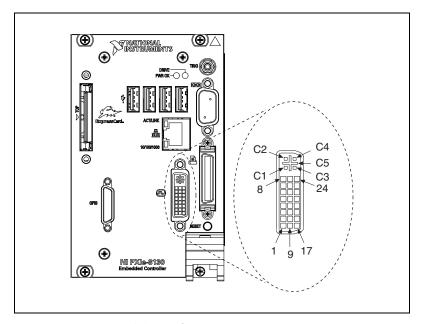
Figure 3-2. DVI Connector Location and Pinout
